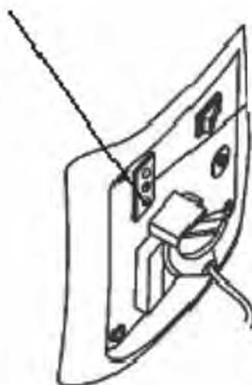
Low oil alarm Indicator Light (Red)
